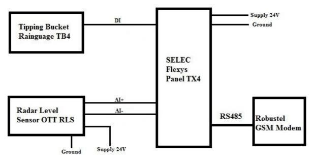
Fig. 1 Connection Diagram of Dam Automation System
